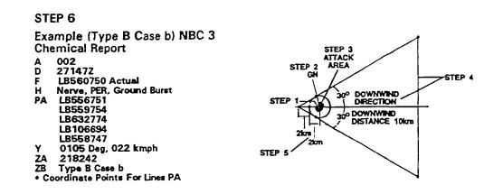
Figure 3-16. Plot for downwind hazard, Type B, Case b.
